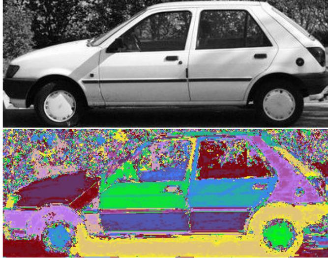
Figure 15: Image segmentation experiment. **Top** The original  $406 \times 158$  pixel image. **Bottom** The segmented image, where different colors represent different segments. The segmentation is solely based on pixel values and the HSNN merges the lower part of the image with the tires of the car. Also, the foliage in the background is segmented with preservation of the texture.
