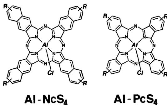
Figure 1. Chemical structure of sulfonated aluminum naphthalocyanine (Al-NcS) and sulfonated aluminum phthalocyanine (Al-PcS).  $R = \text{SO}_3^-$  or H.
